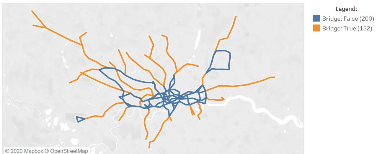
FIG 1. Bridges in the London Underground network. Orange signifies a bridge-link, blue signifies a non-bridge link.
